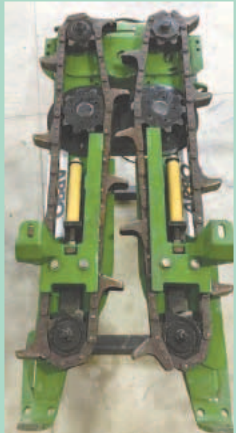
Kopper Kutter kit lets you use a cornhead to harvest crops like sorghum and sunflowers. Kit consists of two 9-in. dia. chain-driven discs with sprockets mounted on back.
