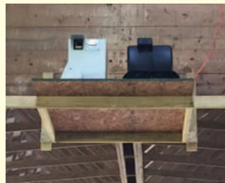
To keep birds out of an 800-ft. freestall dairy barn, an Ohio State University researcher misted Avian Control® Bird Repellent from the rafters with a Bird Buffer Q3 time-release system.
