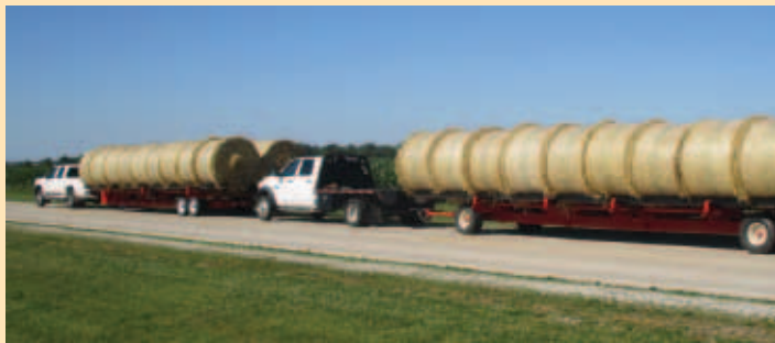
“Lickety-Split” hauler requires no hydraulics or electronics. It’s available in a gooseneck model or a four-wheel-steer model.
