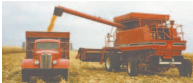
Ewen modified his 1984 combine by adding a Mud Hog axle on back and expanding the grain tank to 300 bu. He likes that the combine doesn’t have all the electronic bells and whistles.
