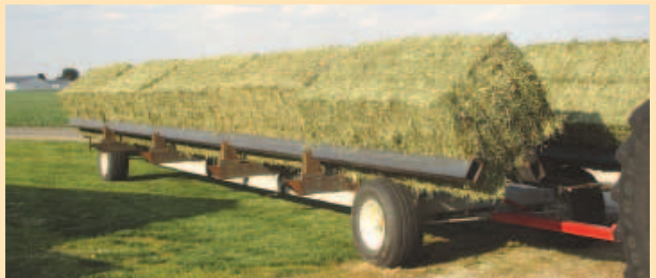
Each cradle consists of 2 adjustable rails made from 4 by 6 rectangular tubing mounted at an angle. Bales can be loaded from the side or rear.
