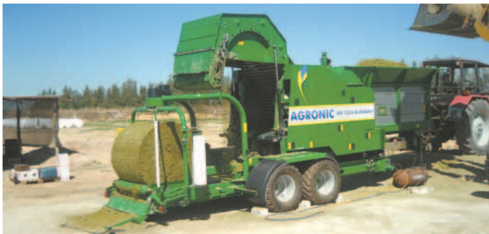
Silage baler can also be operated while stationary, by feeding silage into the hopper from a silo or wagon (above). Baler is made in Finland.
