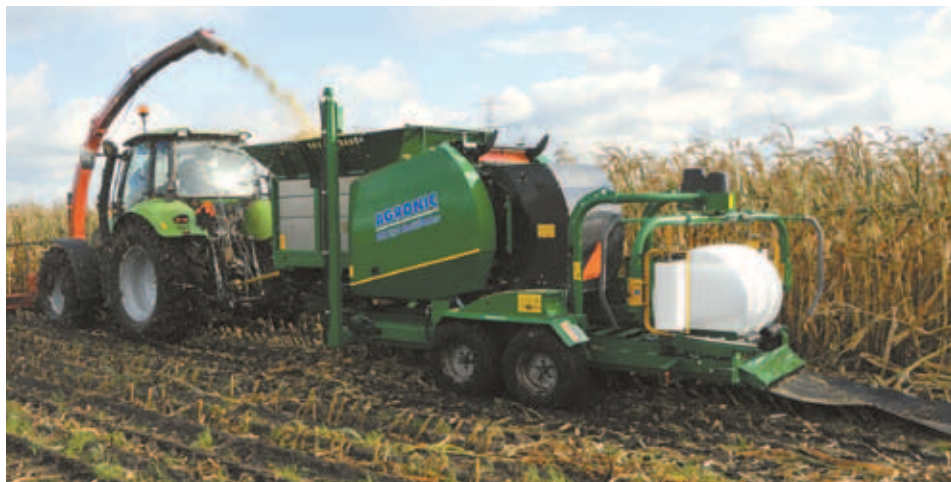
Towed through the field by a forage harvester blowing silage into the hopper, Agronic silage baler compresses and then drops plastic-wrapped bales out the back.
