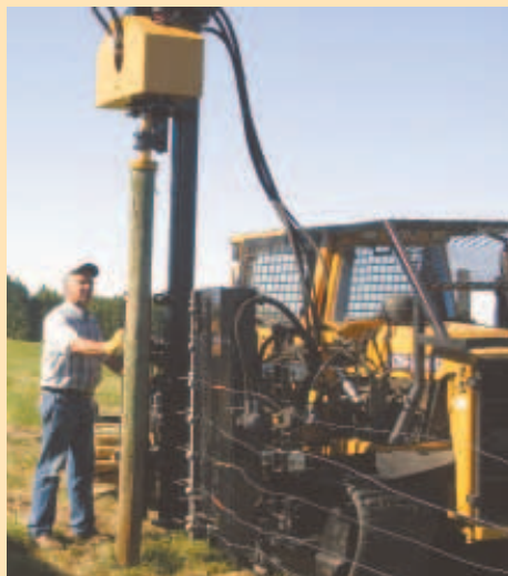
One Pass Fencemaker is a tracked vehicle with a post carrier in front and an automated fencing system attached to its side.
