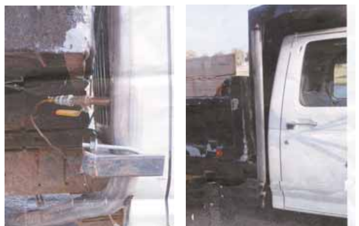
A steel tube runs from a small water tank up through the Ford 350's vertical exhaust stack and then down again. As the water turns to steam, it's pulled through tube and into the air intake between truck's air cleaner and throttle.
