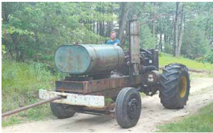
"It does a lot of heavy work. But it's not really a tractor because it can't pull an implement and pto-drive at the same time. I spent less than $5,000 to build it," says Eddie Eron about the self-propelled power unit he built from a junked-out semi truck.
