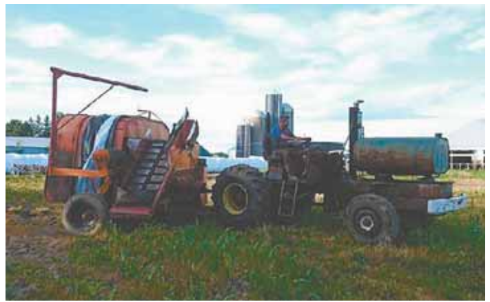
One of the jobs Eron uses the power unit for is to pull a silo bag loader to the bag and then pto-drive it. As the bag fills, the bag loader pushes the power unit along just like with a tractor.
