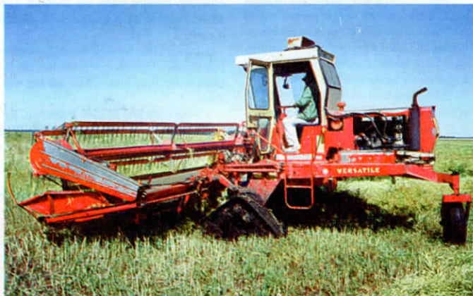
By fitting the tracks on swathers, etc., you can get into wet fields where normal machinery can't.
