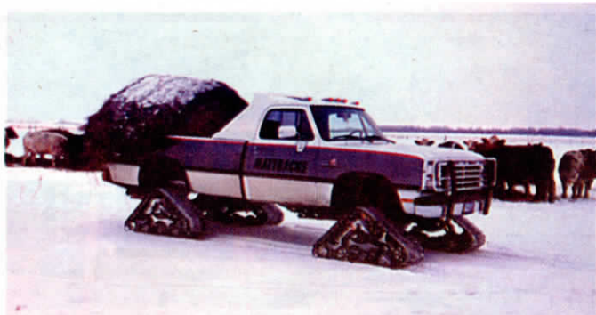
System's four triangular, 16-in. wide tracks add 6 in. of clearance to vehicle.
