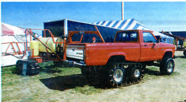
Rubber track kit mounts on pickup. Tandem axle sprayer also has tracks.
