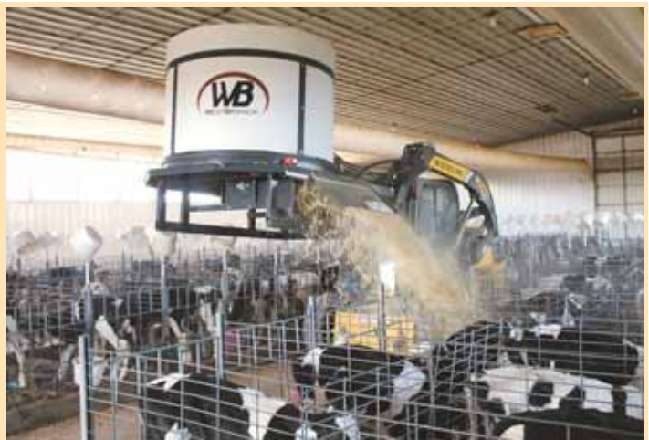
An adjustable deflector blows chopped material out up to 15 ft. or more. "With the chopper mounted on front of the loader, you can drive through freestall pens blowing bedding into the stalls as you go," says Garber.
