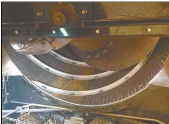
Designed for Class 7, 8 and 9 Case IH combines, Cone Guard requires no modification to the existing transition cone. Once bolted in place, it simply covers any holes or worn areas.
