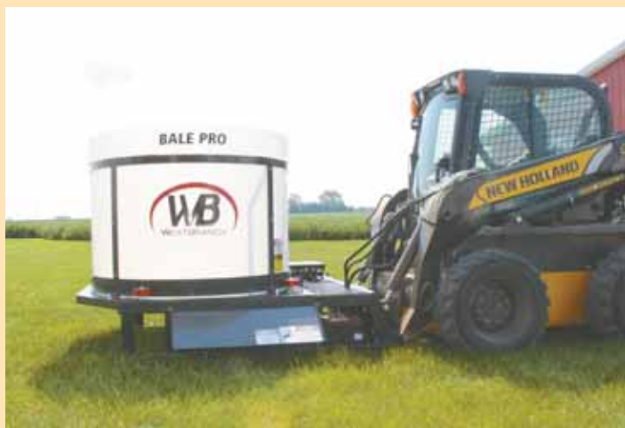
Regan Garber's loader-mounted bale chopper is designed to handle sections of big square bales or multiple small squares. A powder-coated steel frame supports the 52-in. dia. poly tub.
