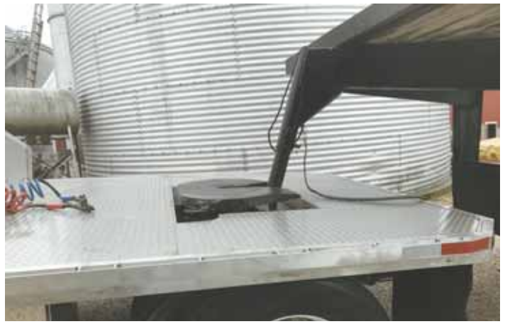
When the 5th wheel or gooseneck hitches are needed, the flatbed deck drops down to allow access.
