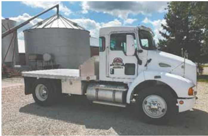
Dan Batdorf needed a flatbed to use around his farm, so he bought an old FedEx semi tractor and fitted it with a 10-ft. long aluminum deck that fits over the 5th wheel.
