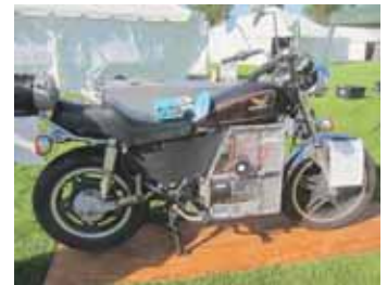
Motorcycle's electric motor is located in front of foot peg. An electric fan mounted beside the batteries keeps motor cool.
