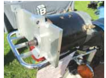
This is the DC motor and adapter that Erdman used to drive motorcycle.
