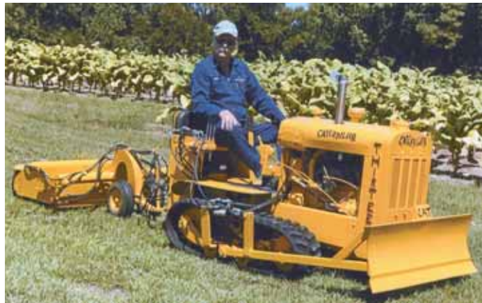
Abe Kemp built this mini bulldozer, blade and dirt pan from scratch. "The dozer has a fully functioning hydraulic blade, and the dirt pan works like the real thing," he says.
