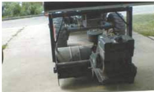
Don Ritchhart bolted a 3-ft. wide garden rototiller to a steel frame that bolts onto his Bobcat's loader bucket. Tiller is powered by a pull-start gas engine.
