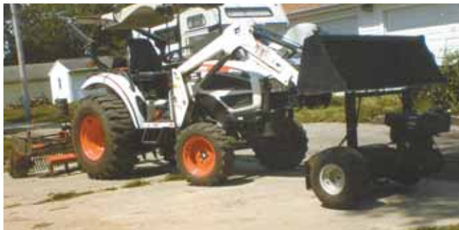
Don Ritchhart bolted a 3-ft. wide garden rototiller to a steel frame that bolts onto his Bobcat's loader bucket. Tiller is powered by a pull-start gas engine.
