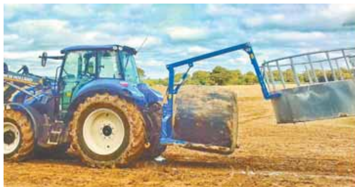
Darragh Egan can haul a bale and bale ring at the same time to a pasture and then lower the ring over the bale, without having to get off the tractor.
