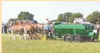
Powered by a 20 hp. engine, litter slinger uses flails with weighted tips to spread material.
