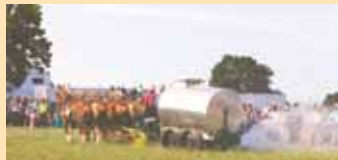
Big tank spreads slurry up to 20 ft., depending on draft team's walking speed.
