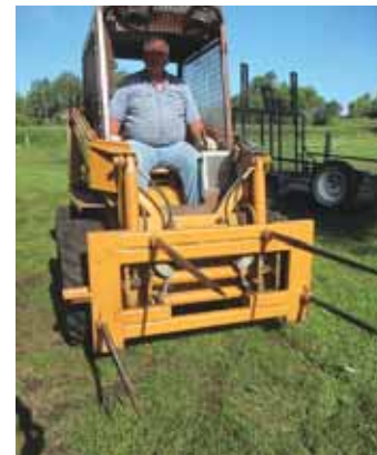
Bale fork consists of four 3-ft. long bale spears mounted on a rectangular steel frame. Large opening in middle of frame provides a good view for the operator.
