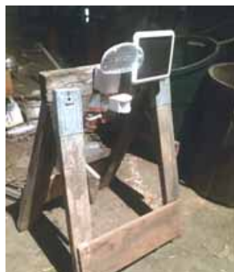
Solar-powered light with motion sensor works great when backing up to an auger hopper at night, and to get rid of varmints.
