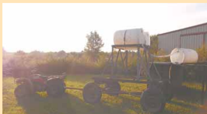
Elevated water tower holds two 55-gal. barrels 6 ft. above base of trailer, high enough to gravity-feed water barrels on rabbit pens.
