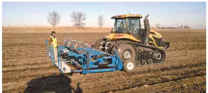
Drip tape was installed by a special machine using RTK guidance on the tractor.
