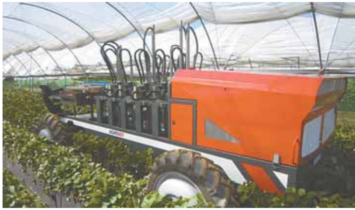
Agrobot machine from Spain uses cameras to identify ripe fruit.
