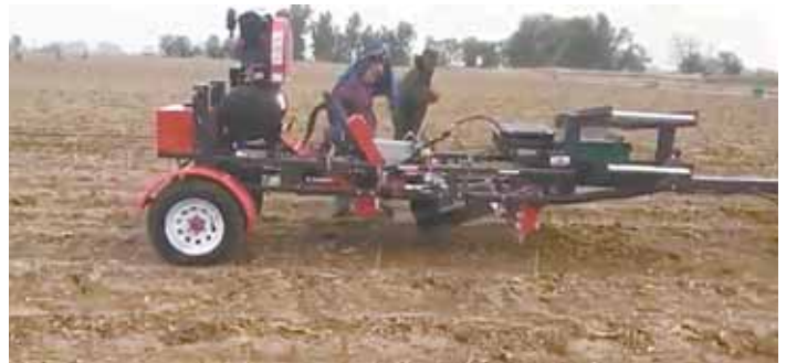
Asparagus picker has electronic eyes and mechanical arms with cutting blades. It senses spears that are tall enough to harvest, then grips, slices and conveys them into a box.
