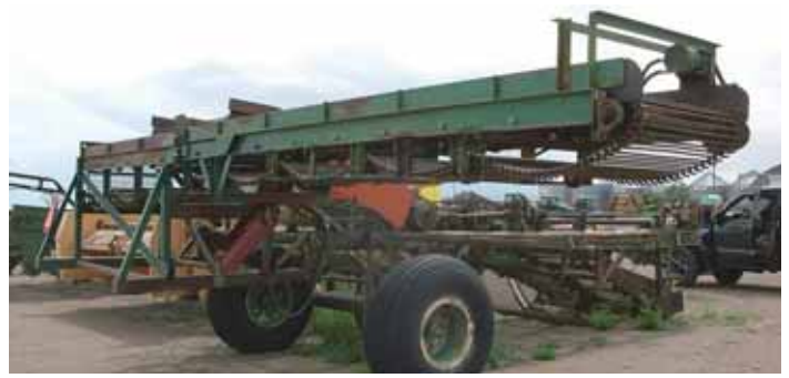
Side-mounted conveyor on back raises and lowers hydraulically to dump rocks into a semi trailer.
