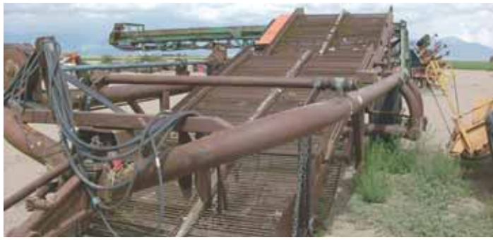
Trailing rock picker was built out of a Grimme potato harvester and a 4-row Lockwood potato windrower. A pair of pto-driven, 30-in. wide chain conveyors ride on top of rollers.
