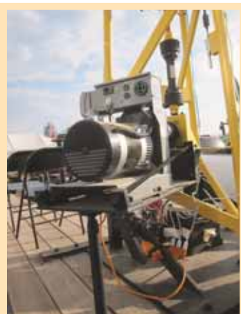
Phoenix windmill produces AC electricity. Fan assembly and tail drives a gearbox and driveline, which in turn chain-drives a generator.
