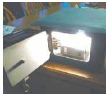
Steel box encloses a thermostat and porcelain light fixture for a 60-watt light bulb. A plastic waterer sets on top of box and is warmed by its top plate.
