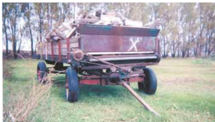
Roger Reibsamen built this self-unloading trailer out of a chopped-down silage wagon. It unloads out the back using the original apron chain.
