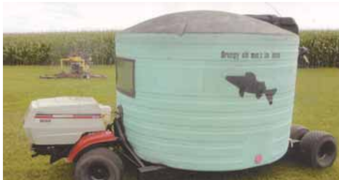
A 1,000-gal. poly water tank bolts to the extended undercarriage of an old lawn mower.
