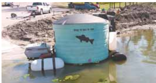
A 1,000-gal. poly water tank bolts to the extended undercarriage of an old lawn mower.
