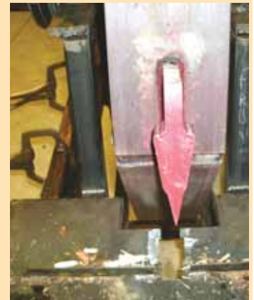
As wheel rotates the axe head comes down on top of log, splitting it in half.
