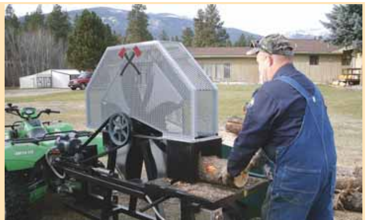
Flywheel log splitter consists of a heavy spinning steel wheel with a welded-on axe head that revolves continuously and goes through a slot cut into table.
