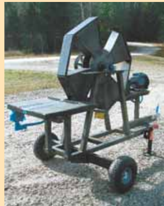
As wheel rotates the axe head comes down on top of log, splitting it in half.
