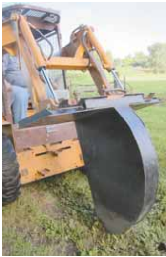
Trencher's rounded steel bucket is welded onto a quick-tach mounting plate. A pair of carbide steel teeth spaced 6 in. apart weld to front edge.
