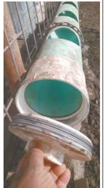
Trough is made from a heavy-duty pvc pipe with screw-on caps on the ends. Cut-outs allow pigs to access the water.
