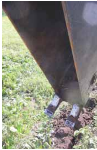
Trencher's rounded steel bucket is welded onto a quick-tach mounting plate. A pair of carbide steel teeth spaced 6 in. apart weld to front edge.
