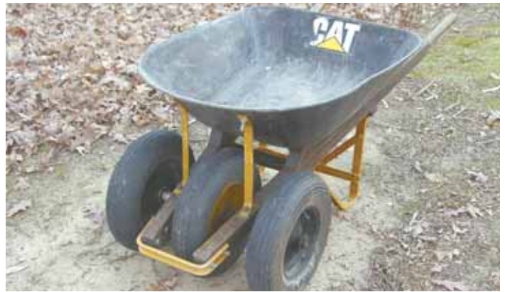
Billy Gilbert made his wheelbarrow more stable and increased its hauling capacity by adding 2 matching wheels on front.
