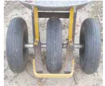
Wheelbarrow's original axle was replaced with a long steel rod. Electrical conduit spacers separate the wheels.
