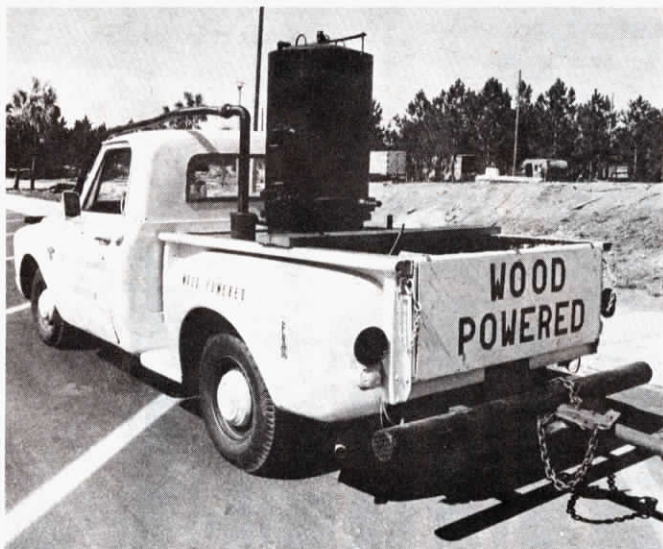
1967 Chevy pickup generates its own fuel "on the go" with wood burning generator mounted behind cab.
