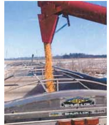
Spring-loaded spout can be adjusted forward or backward by cranking a hand-operated winch at bottom of auger.
