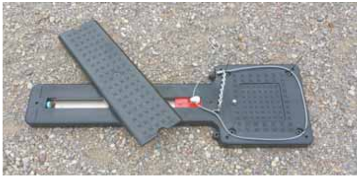
Select-A-Catch foot snare can be set for the weight of the animal to be caught. A 12-in. square tension pad with a 6-in. square trigger at the center activates the snare.
