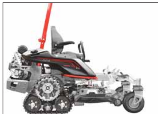
TRX tracked zero-turn mower has front suspension and rear torsional suspension to provide a smooth ride. The company says it can go where traditional zero-turn mowers can't.
