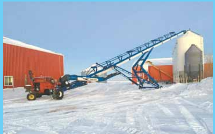
Andy Steinberger uses an old self-propelled New Idea Uni-Harvester power unit to operate and move his big 20-in. wide, 110-ft. long belt conveyor.
