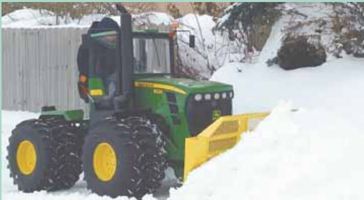
Don Campbell started out with the frame, axles and engine from an old Steiner front-mount riding mower to build this half-scale articulating Deere 9630 4-WD tractor.
