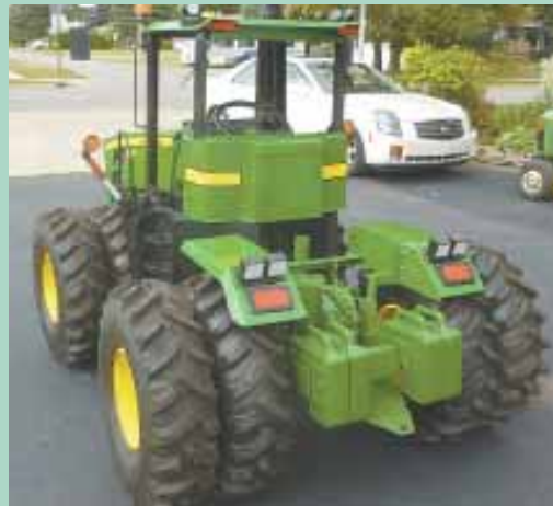
He lengthened the mower's front and rear frames and made new fenders, fuel tank, and hood. "The cab is proportional to the tractor. It looks factory-built," says Campbell.
