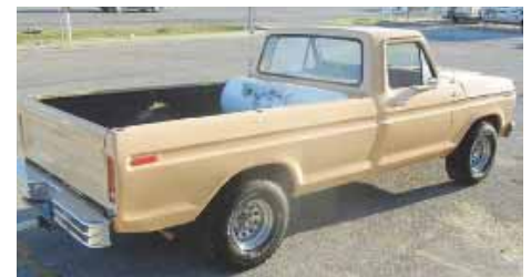
Steve Edwards of Granbury, Texas, says he couldn't be happier with his 1978 propane-powered Ford F-150 pickup. It has more than 576,000 miles on it.
