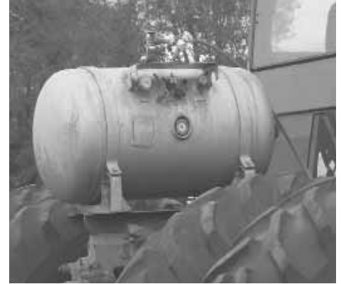
Propane Enhancer injects a little propane into diesel engines for faster speeds, more power, and a cleaner burn in tractors and trucks.
