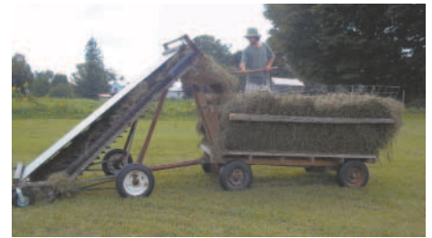
Gies bought an 18-ft. long, 4-ft. wide hay loader, reversed the belt direction, and mounted it in front of a wagon. He mows, rakes and loads 6 acres of hay 3 times every summer.
