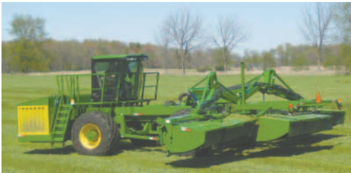
Self-propelled mower conditioner is equipped with three 16-ft. cutting and conditioning heads.
