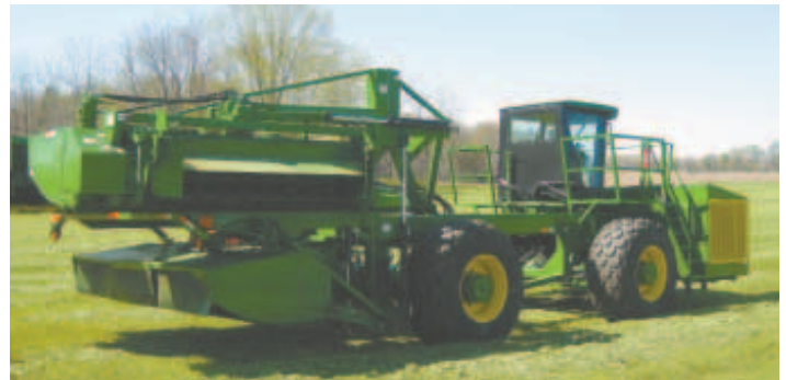
Machine’s Deere cab mounts on a manual turntable, allowing the operator to drive forward both in the field and on the road. Cab can be turned 180 degrees for transport.
