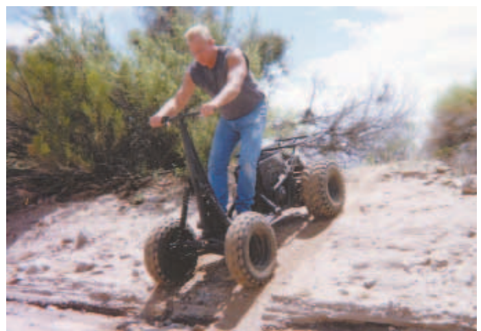
The 4-wheeler's front and rear ends have independent frames connected at a pivot point. "The front end can twist one way and the back another," says Zuhlsdorf.
