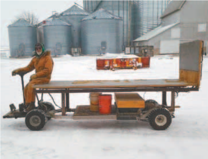
Paul Butler converted a Club Car 6-passenger, electric-drive golf cart into this “big bale cart” that handles big square bales weighing up to 800 lbs.
