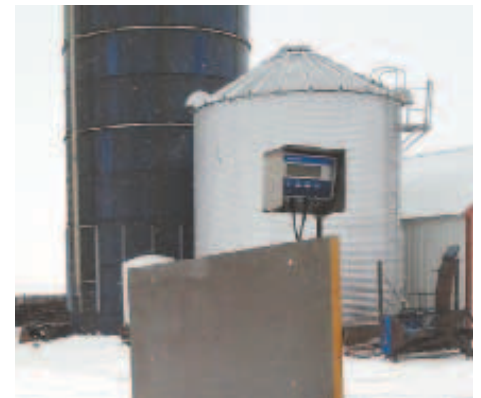
Electronic weigh scale mounted on back of cart shows bale’s weight.
