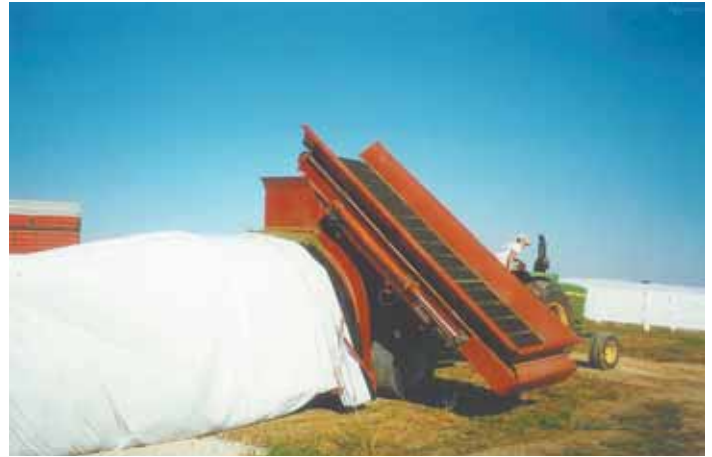
Pto-operated RamPack silage bagger uses dual plungers to fill a plastic forage bag, instead of a rotor or auger. Developers say it will speed up the process of bagging.
