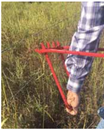
Hinged tool has 2 handles, both fitted with rows of interlocking teeth that form a "jaw" over wire. Operator pushes top half of tool down through bottom half to crimp the wire, then raises it back up to release wire.
