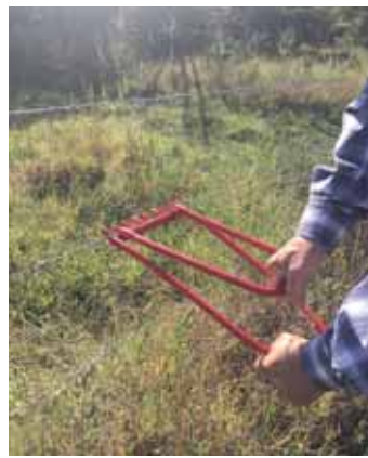
Hinged tool has 2 handles, both fitted with rows of interlocking teeth that form a "jaw" over wire. Operator pushes top half of tool down through bottom half to crimp the wire, then raises it back up to release wire.
