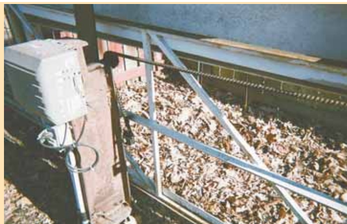
Pushing the button on the remote control opener engages the jackshaft to slide gate open or shut.
