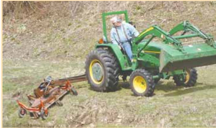
Add-on boat winch lets Joe Bowers lift his swivel sidearm mower vertically to cut shrubs and bushes or drop it down to mow ditch banks.
