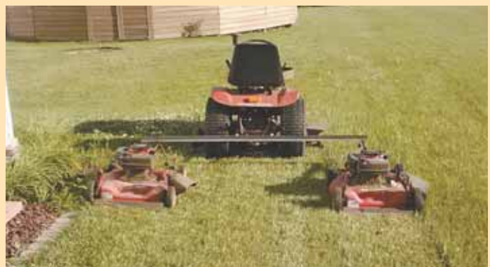
Rob Ribar built this hitch to pull two 22-in. push mowers behind his Wheel Horse riding mower. The 3 decks cut an 88-in. wide swath.
