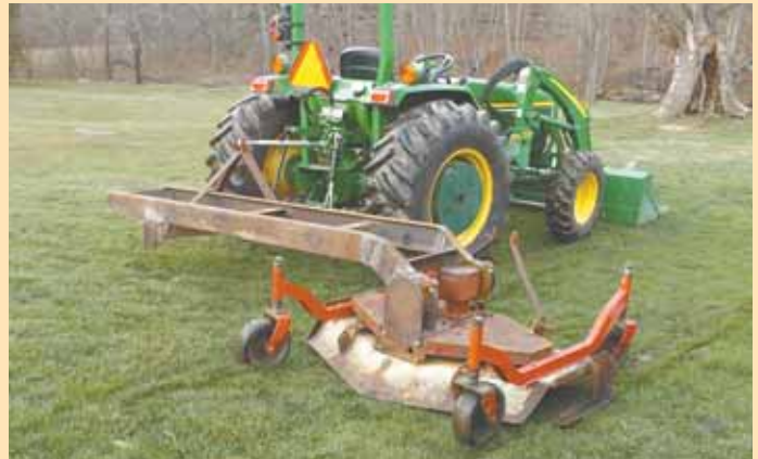
Mower hooks up to the 3-pt. hitch on Bowers' Deere tractor. He uses it to mow 2,000 ft. of creek bank.
