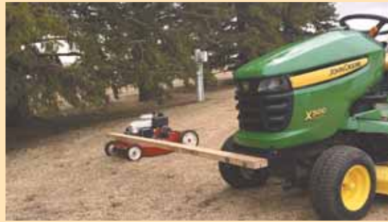
Attaching a push mower to an 8-ft. long 2 by 4 lets Charles Anderson mow under evergreen trees.
