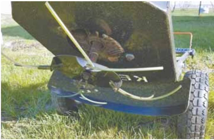
"It has an open deck that doesn't plug up with wet grass like a regular push mower," says Dan Kern about his 3-wheeled, 22-in. wide string mower/trimmer. It uses the largest trimmer string line on the market.
