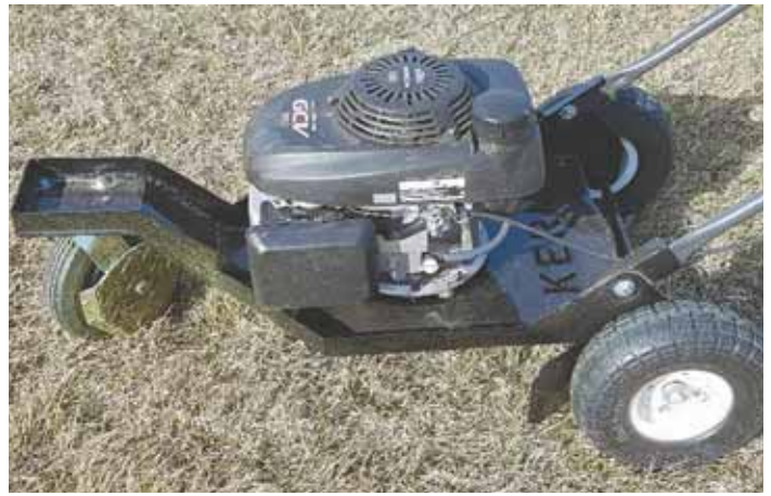
Trimmer's front caster wheel makes it more maneuverable than a 2-wheeled string trimmer, says Kern.
