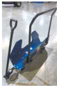
You tilt the cart and scoop to load animal, then pull cart upright and wheel it away.
