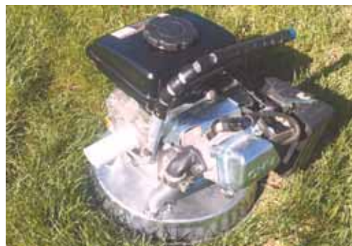
"Predator Gopher Killer" uses a 3 hp., 4-cycle gas engine mounted above an inverted steel pan to kill rodents with carbon monoxide.
