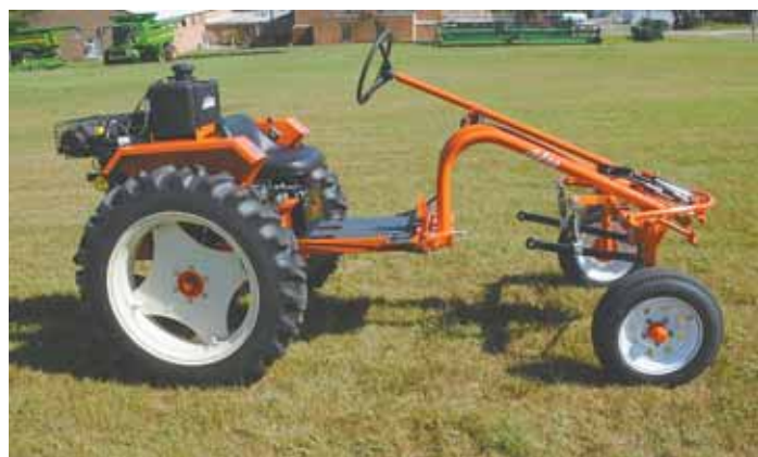
Tuff-bilt tractor can be powered by either a fuel-injected gas engine or a diesel engine.
