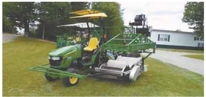
Leon Perry's home-built wild blueberry harvester is built on a subframe that runs directly behind the tractor, instead of out to the side, to avoid driving over blueberries.
