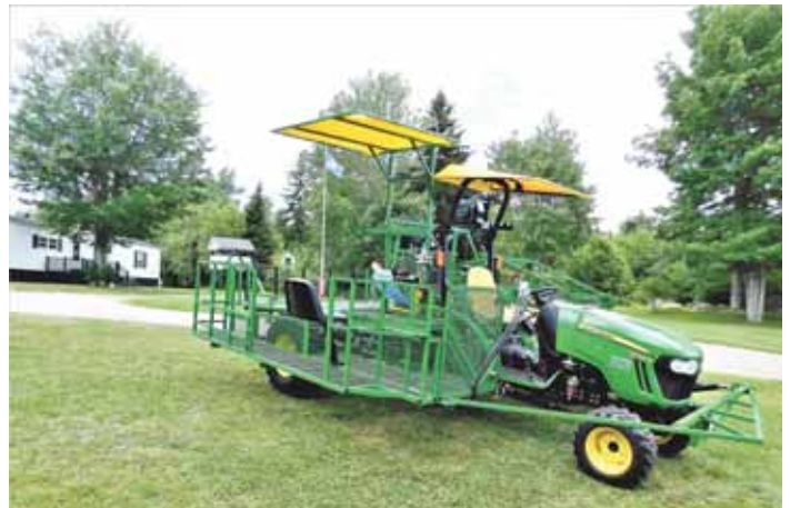
To support the subframe, Perry removed the wheels from tractor's rear axles and moved them 7 ft. back onto individual axles.
