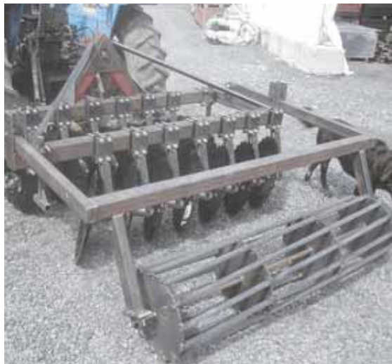
A farm group in Quebec get together to design and build equipment for smaller farms. They recently put together this 3-pt. mounted tillage tool called an oblique disk cultivator. It's similar to ones used in Europe.
