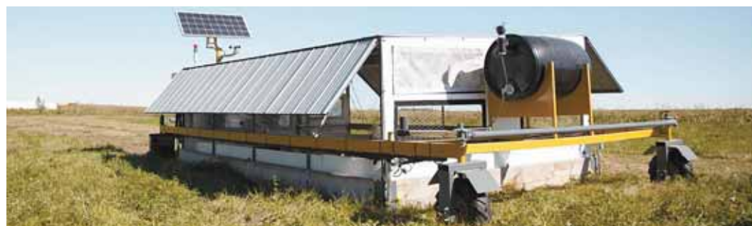
Solar-powered robotic chicken coop moves automatically and carries a week's worth of feed and water. It can be controlled from a smartphone. "Because it's fully automated, I spend only 5 to 10 min. a day checking on my chickens," says Daniel Badiou.
