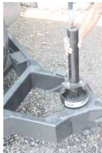
Trailer jack slips through Jack-E-Up device, which engages jack when cranking to lift and lower trailer.
