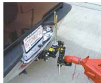
Reel-Quick Hitch extends hitch ball rearward, to hitch up. Hand crank pulls it back in.
