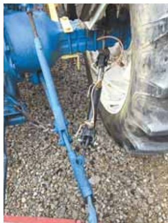
A pair of ball valves mount on the cylinder ports. "I close the valves wherever I want the lift arms to be, and they stay put," says inventor Larry Wood.
