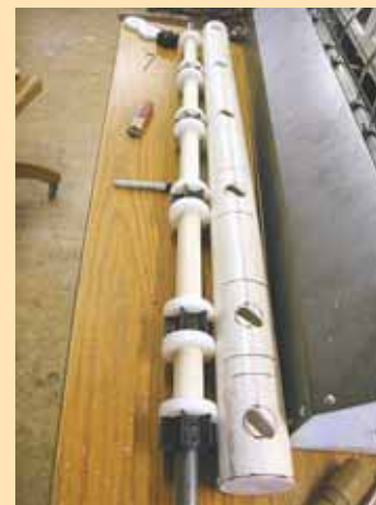
“Agitation” shaft runs through drill hopper and is ground-driven by a sprocket mounted on disc gang shaft (left). Drill’s seed metering system fits inside a 2 1/2-in. pvc tube.
