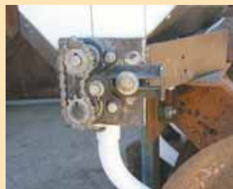
Photo at left shows secondary drive to metering shaft. Photo at right shows metering tube attached to bottom of hopper.
