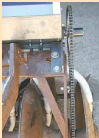
“Agitation” shaft runs through drill hopper and is ground-driven by a sprocket mounted on disc gang shaft (left). Drill’s seed metering system fits inside a 2 1/2-in. pvc tube.
