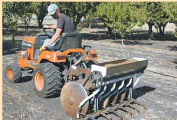
Bill Spurlock built this 3-pt. mounted disc drill on the single front gang off an old disc harrow. He uses it with his compact Kubota BX1500 tractor.
