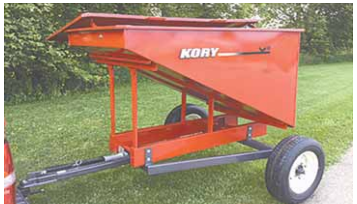
Kory 1-ton gravity wagon has a formed steel lid and a rear discharge for filling feed pails. Works great to haul corn for corn-burning furnaces, as well as wood pellets.
