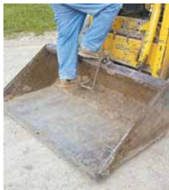
A 12-in. metal step attached to top edge of bucket makes it easier for Chuck Virtue to climb into his skid loader. A cotter pin holds step in place.
