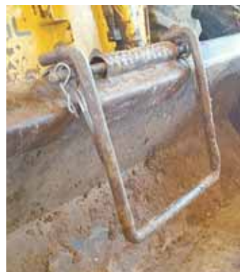
A 12-in. metal step attached to top edge of bucket makes it easier for Chuck Virtue to climb into his skid loader. A cotter pin holds step in place.
