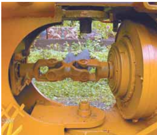
Gerald Sundberg built this 4-WD articulated log skidder out of 2 Farmall F12 rear ends and an Allis Chalmers WC engine and transmission. The rear ends face each other and are connected by a shaft and double U-joints.
