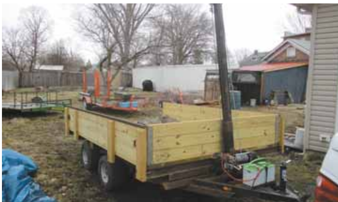
Steve Nichols built this dual axle dump trailer, mounting a 10,000-lb., 12-volt winch equipped with a remote control on front. Box dumps at a 55 degree angle.
