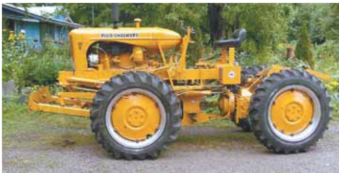
Gerald Sundberg built this 4-WD articulated log skidder out of 2 Farmall F12 rear ends and an Allis Chalmers WC engine and transmission. The rear ends face each other and are connected by a shaft and double U-joints.
