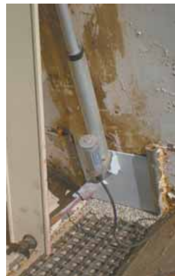
Ben Taylor used about $100 worth of parts to build a variable-rate controller for his dry fertilizer spreader.
