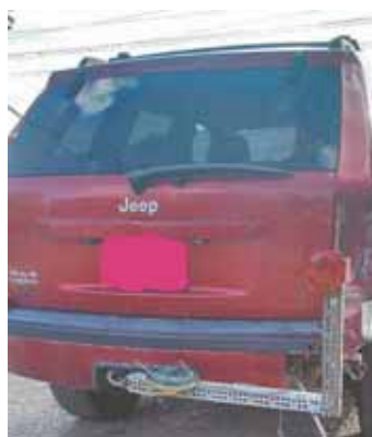
When his wife's Jeep got rear ended, Glenn Haley used a trailer light kit to keep the vehicle going until the damaged area could be repaired.
