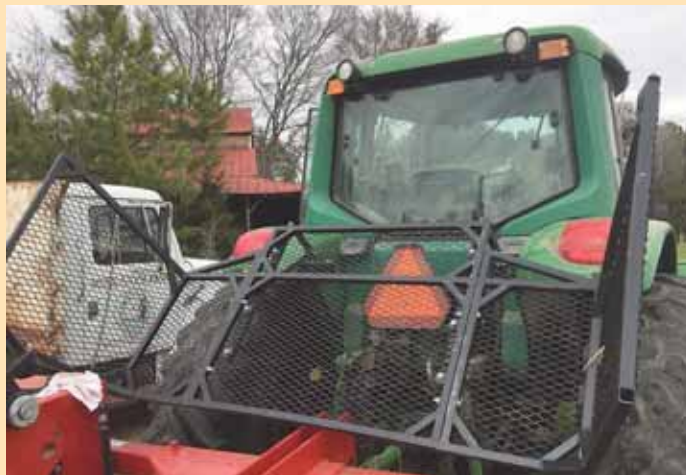
Standard screens are designed to protect tractor cab rear windows. Screen shown here, custom built for a Deere 7220, also extends forward to protect side windows.
