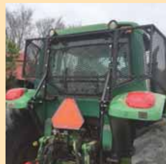
Standard screens are designed to protect tractor cab rear windows. Screen shown here, custom built for a Deere 7220, also extends forward to protect side windows.
