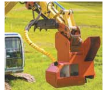
Ditch Doctor mounts on the arm of a 13 to 22-ton excavator. Its rotary head can throw material up to 120 ft. across a field in self-leveling deposits.
