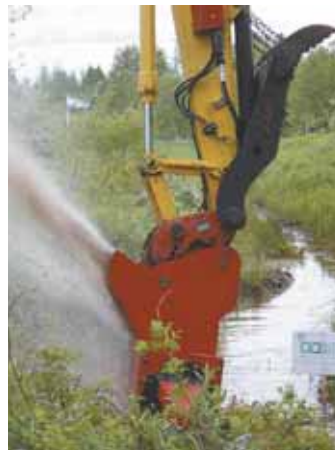
Ditch Doctor mounts on the arm of a 13 to 22-ton excavator. Its rotary head can throw material up to 120 ft. across a field in self-leveling deposits.
