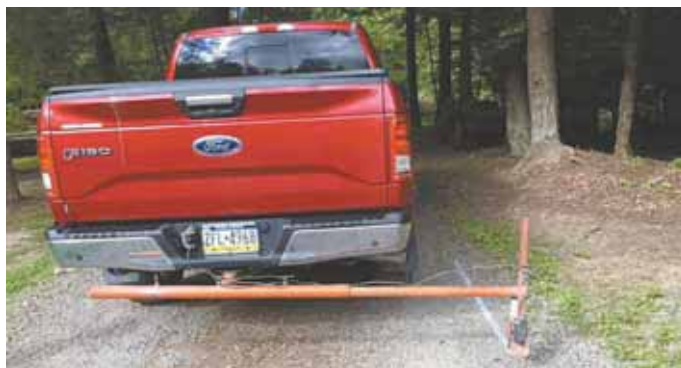
Made of metal tubing, Phillip Ackley's line painter mounts on a 2-in. hitch receiver and is powered by a trailer plug-in.
