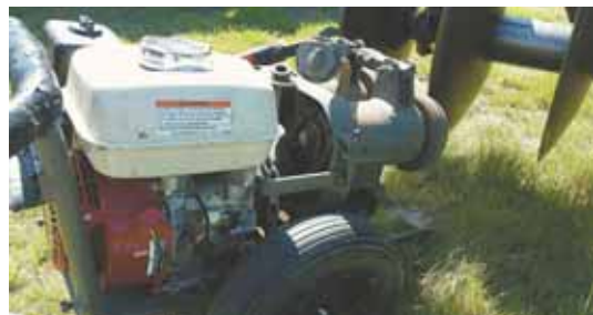
Jess Putnam uses this disc blade roller to roll the edges on disc blades. He says the process adds years to disc blade life.
