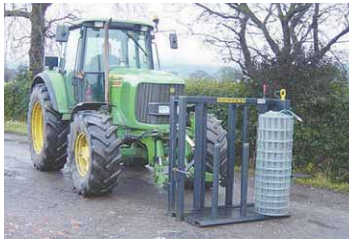
Quickfencer mounts on front or rear Cat. III 3-pt. hitches to simplify installing woven, bare or barbed wire fences.
