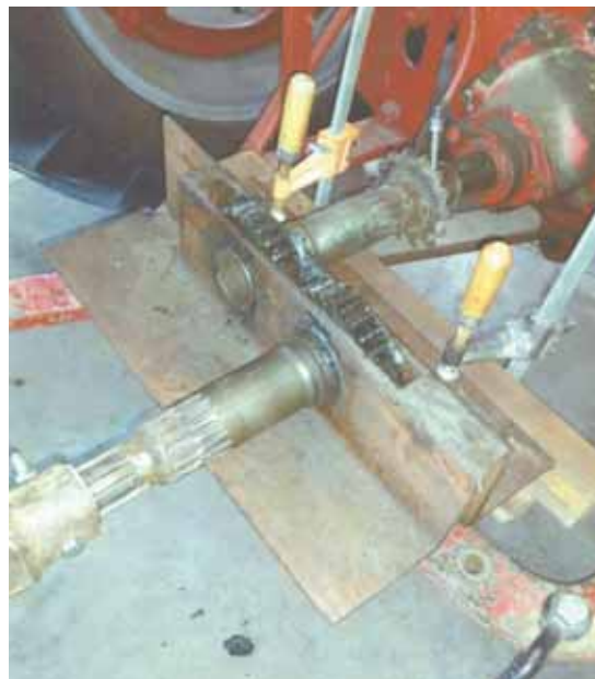
Loren Eddy's pto reverser uses 2 gears left over from live power units in older IH tractors. "It does a neat job of breaking in a newly overhauled engine," says Eddy.
