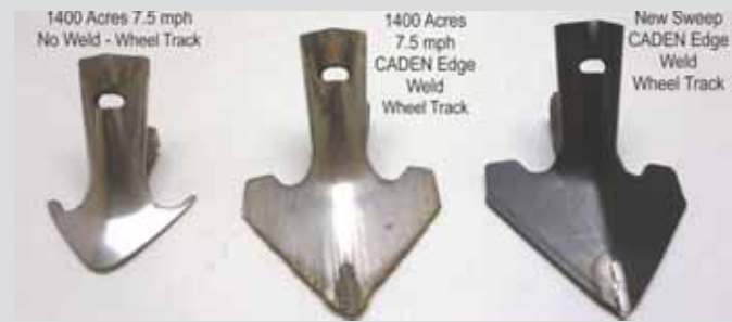
CADEN’s hard-surfaced “Wheel Tracker” field cultivator shovels are made with an ultra-tough surface that resists abrasion for long wear.
