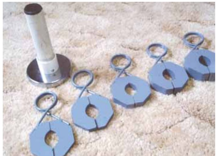
Hexagon-shaped steel stop blocks come in 2 pieces that pull apart using a coil spring welded onto one side. "My Steel blocks hold up much better than aluminum," says Roger Kuntz.
