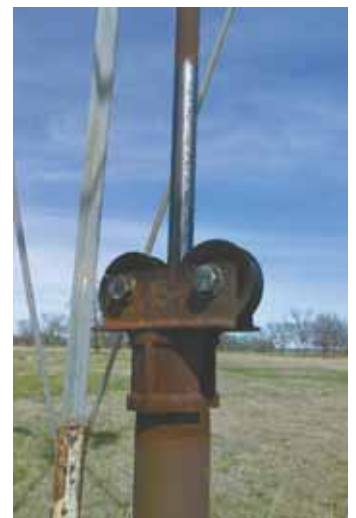
A pair of plastic pulleys keep windmill's sucker rod perfectly centered inside well pipe.
