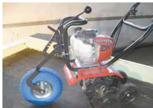
Machine builds raised rows that remain year around. Excess rain is held in row middles instead of running off.
