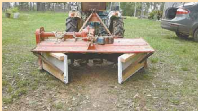
Metal wings on back of tiller extend out from both sides of tiller housing to form raised bed.
