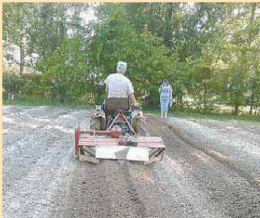
Metal wings on back of tiller extend out from both sides of tiller housing to form raised bed.
