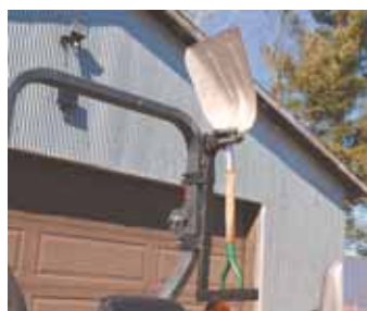
Tool holder bolts onto one side of ROPS and uses plastic ratchet-type clamps to hold tool in place.
