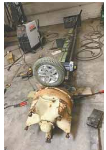
Rubber drive wheel at top of upright friction-drives the hub on a military trailer axle to rotate swing.
