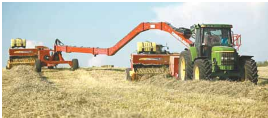
Swing Max dual baler hitch keeps the first baler on path with the tractor, while hydraulic control from the cab directs the second baler.
