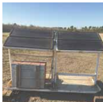
Portable solar-powered setup provides pond water to Cox's cattle. Four 40-watt solar panels are wired to a pair of 12-volt batteries located inside box on platform.
